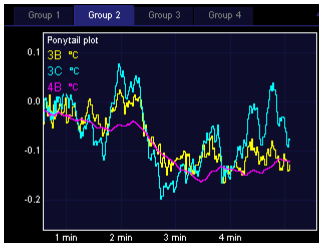
In ponytail plot mode, all traces are offset so that they start at zero.
