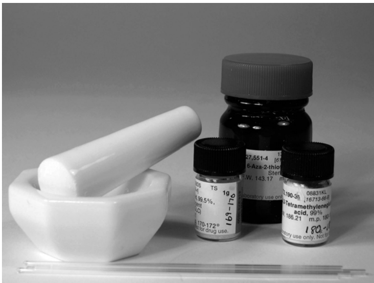
Solid samples, mortar and pestle, and capillary tubes—the basic ingredients for sample preparation.
