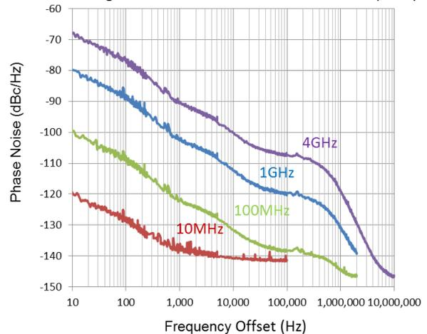
SG396 Single Sideband Phase Noise vs Offset Frequency
