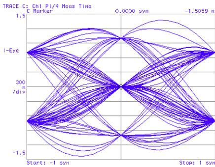
NADC I-Eye diagram (875 MHz carrier)
