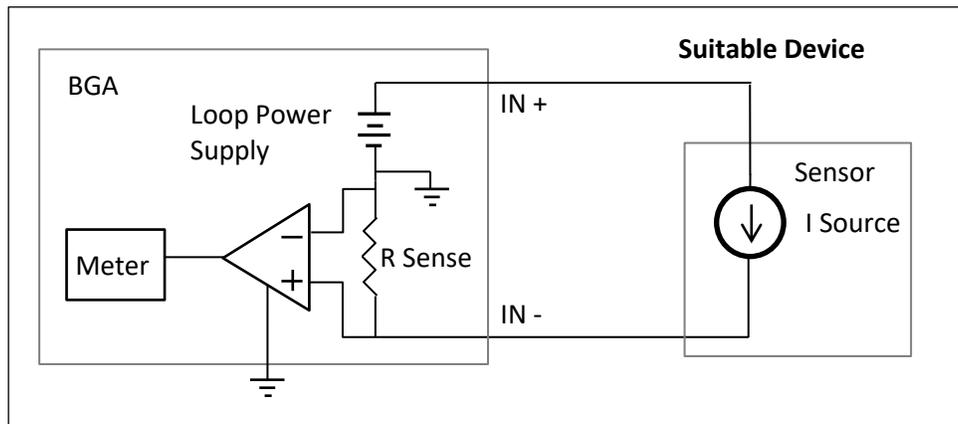
FIGURE 9: CURRENT INPUT W/ LOOP POWER (SUITABLE DEVICE)
