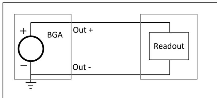
FIGURE 5: VOLTAGE OUTPUT
