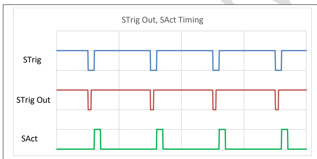
FIGURE 13: TRIGGER AND FLAG TIMING
