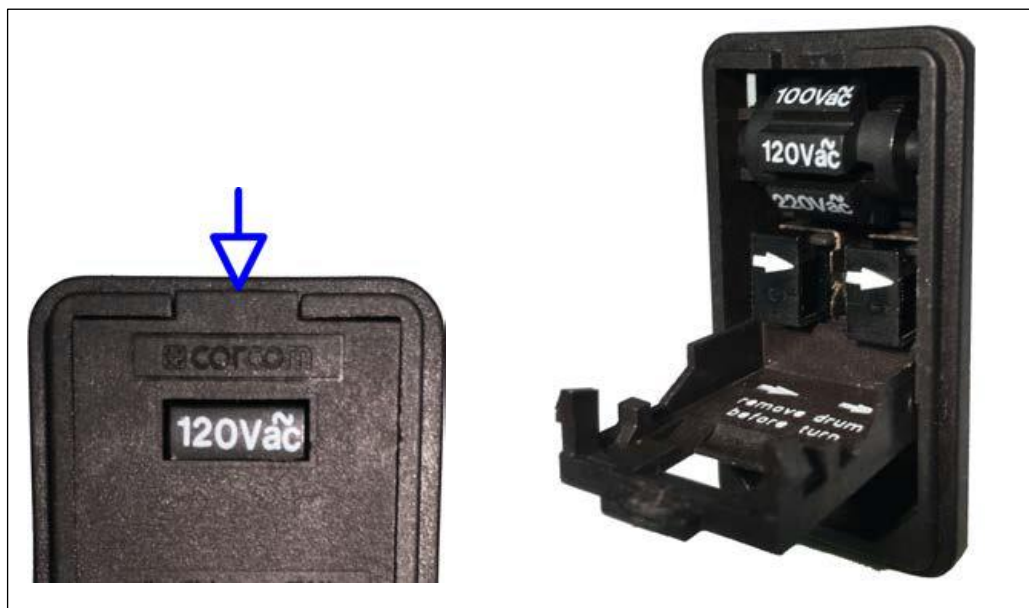
FIGURE 36: POWER ENTRY MODULE VOLTAGE SELECTOR
