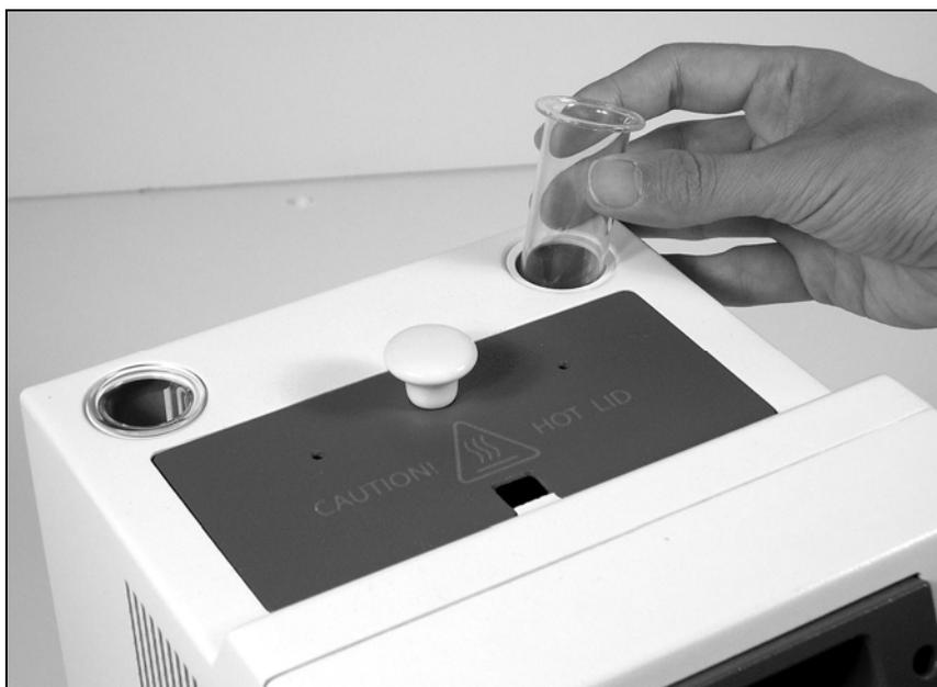
Figure 3. Mounting the glass Capillary Holders.
