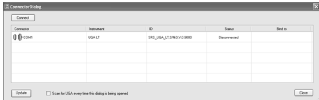
Fig. 2-14. Screenshot of UGA control software after selecting 'Connect' in the 'Main' menu. The available serial connector is shown.
