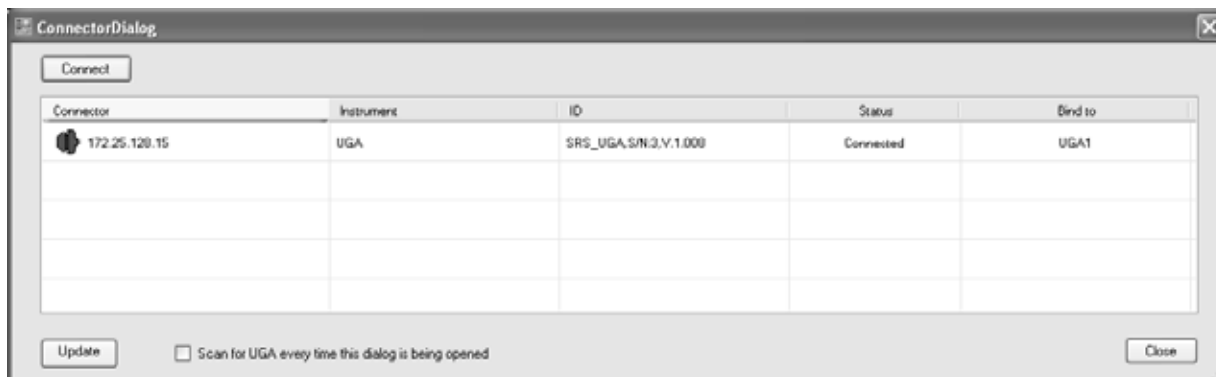
Fig. 2-11. Screenshot of the 'ConnectorDialog' window after proper connection.
