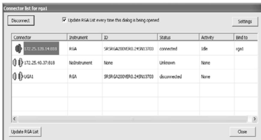
Fig. 2-28. Screenshot of RGA connection dialog box for Ethernet.
