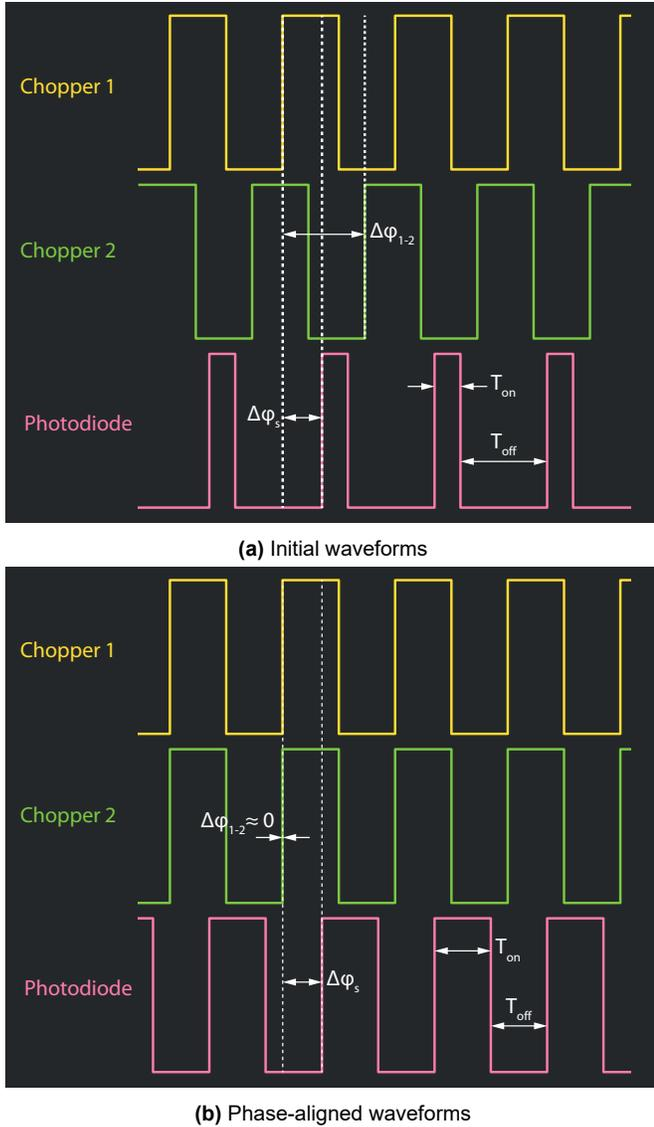
**Figure 5:** Simulated oscilloscope traces for a beam passing through a series of two optical choppers. (a) Before phase alignment, a phase shift  $\Delta\phi_{1-2}$  exists between the chopper 1 and chopper 2 signals, and the photo-detector signal duty factor ( $T_{on}/T_{off}$ ) will likely be  $<50\%$ . (b) After phase alignment, the photo-detector output waveform has a 50% duty factor. The phase shift  $\Delta\phi_s$  of the photo-detector signal persists.
