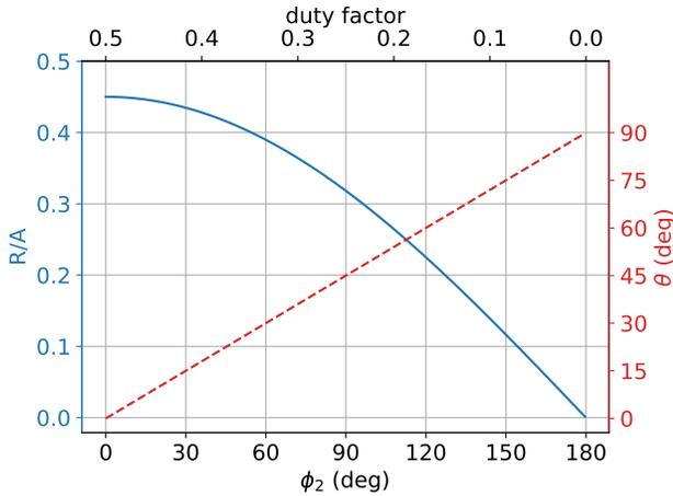
**Figure 8:**  $R$  (normalized to square wave peak-to-peak amplitude  $A$ , and including the factor of  $1/\sqrt{2}$  for RMS) and  $\theta$  vs.  $\phi_2$  (chopper 2 phase) and duty factor, for lock-in harmonic  $n = 1$ .
