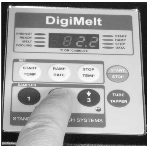
Flagging a point during the melt
