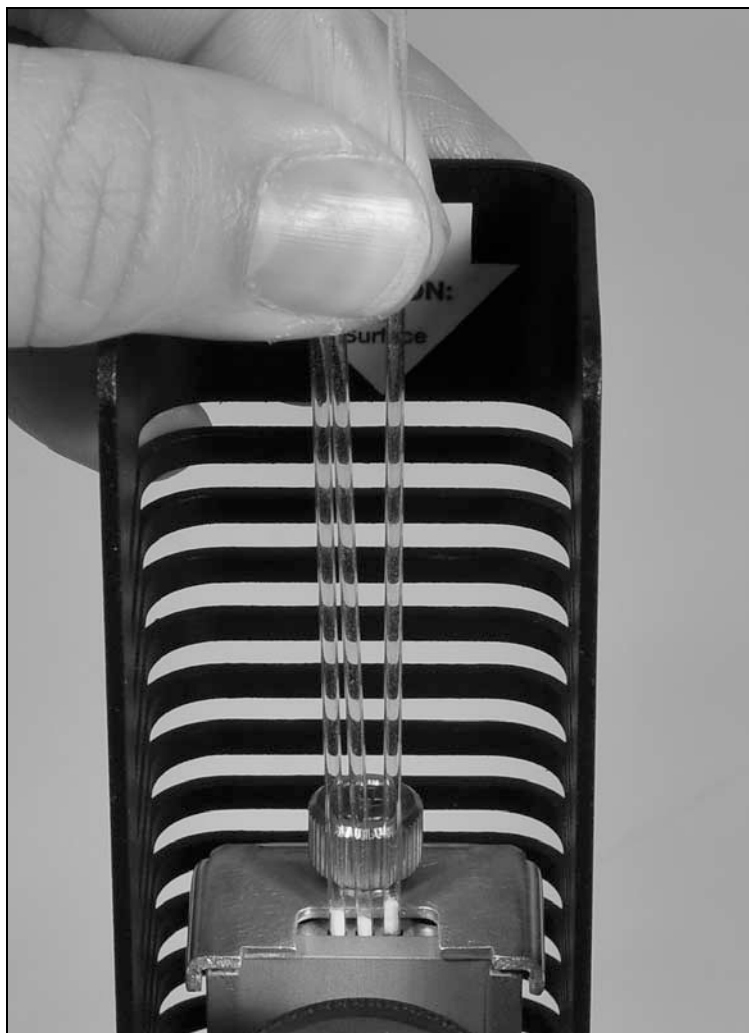
Loading capillaries into DigiMelt.
