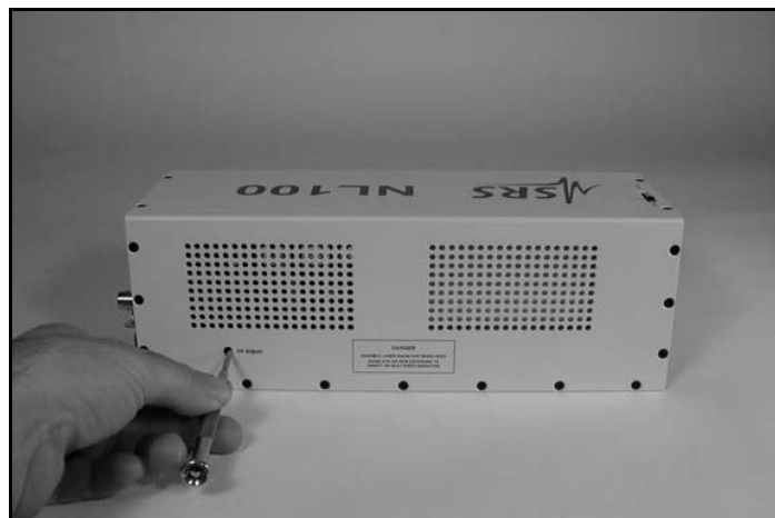
Figure 17. Changing the high voltage adjustment potentiometer.
