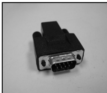
Figure 8. Supplied interlock defeat connector.
