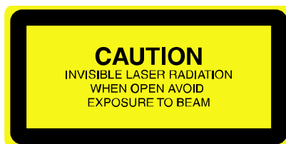
Figure 6. Caution label, located on both sides of the protective cover.
