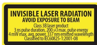
Figure 4. Invisible laser radiation label, located on the side of the protective cover
