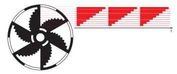
**Figure 3:** O542DF variable duty factor blade. Depending on the beam position along the blade radius, the duty factor can be set to  $n \times (10\%)$  (for n = 1, 2, 3...9).
