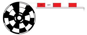
Figure 1: The O54256 5/6 dual-slot blade modulates an optical beam with 50% duty factor:  $T_{\rm on} = T_{\rm off}$ .
