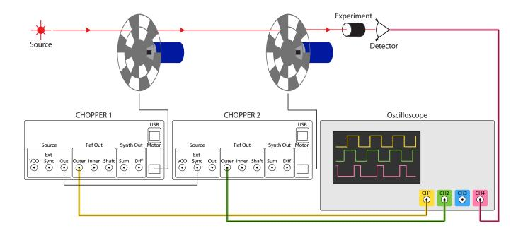
**Figure 4:** Block diagram for synchronization and phase alignment of two SR542 Optical Choppers using an oscilloscope. Chopper 1 is the primary timekeeper, so it's Source Output is connected to Chopper 2's Ext Sync Input. Outer Slots Reference Outputs from both choppers are connected to an oscilloscope, as is the dual-chopped beam signal, which is output from a photo-detector.
