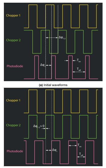
(b) Phase-aligned waveforms
