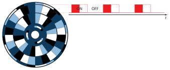
**Figure 2:** A 25% duty factor on the outer track can be achieved by stacking a second blade (shown in transparent blue), with a relative rotation of  $90^{\circ}$  opt ( $15^{\circ}$  mech). Original 50% duty factor is shown with red dashed line for reference.
