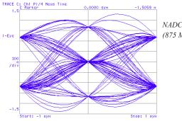
NADC I-Eye diagram (875 MHz carrier)
