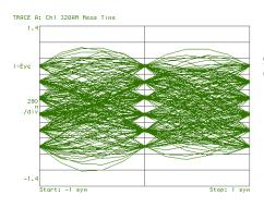
QAM32 I-Eye diagram (5.8 GHz carrier)
