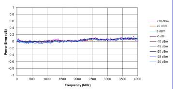
SG396 power error (-30 dBm to +10 dBm, DC to 6 GHz)
