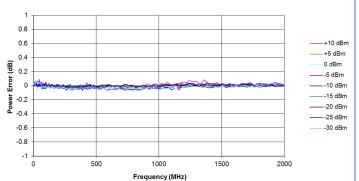
SG394 power error (-30 dBm to +10 dBm, DC to 4 GHz)
