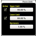
The Upper Limit must be greater than the Lower Limit and within the operating range of the measured parameter. If not, an "Invalid Entry" message will appear with guidelines for a legal value.
