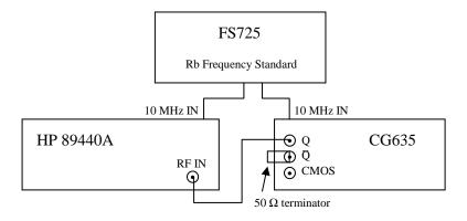
Figure 10: Setup for phase noise and jitter tests.
