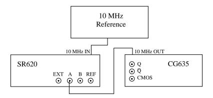
Figure 11: Setup for timebase calibration
