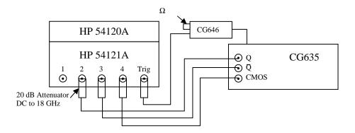
Figure 6: Transition time measurement setup
