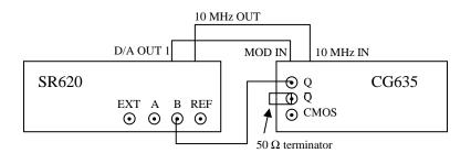
Figure 9: Setup for time modulation test.
