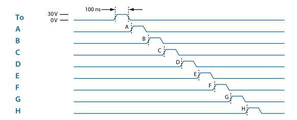
Figure 5: Option 2 Rear Panel Outputs vs Programmed Delay
