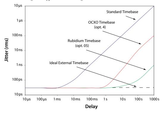
Figure 3: Typical rms Jitter vs. Delay Setting
