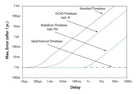
Figure 2: Typical DG645 Timing Error 1 Year after Calibration
