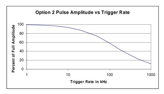
Figure 6: Option 2 Amplitude Reduction vs. Trigger Rate
