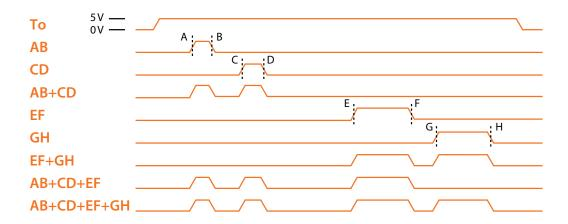
Figure 7: Option 3 Rear-Panel Outputs vs. Programmed Delay
