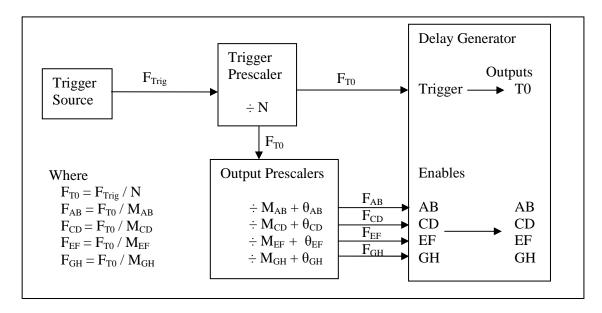
Figure 10: The DG645 Trigger Prescaling
