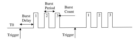
Figure 11: T0 Output in Burst Mode
