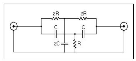
Figure 5-1 Twin-Tee Notch Filter
