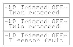
Any of these messages indicate the laser diode driver has tripped off because of a temperature limit setting. Note that these conditions can operate even when the TEC is off, as long as a valid temperature sensor is connected.
