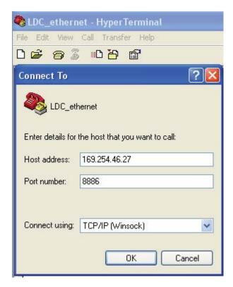
After clicking "OK" in the "Connect To" window, you should see the following message from the LDC500 displayed by HyperTerminal.
