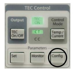
Figure 3.7: The TEC configuration menu selection.
