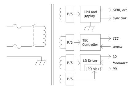
Figure 1.1: The LDC500 power supply block diagram.
