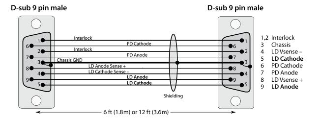
Figure 6.1: Laser diode cable with mating connector. SRS part number O500C3 (6 ft) or O500C5 (12 ft).
