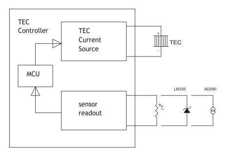
Figure 1.3: The TEC controller (simplified).
