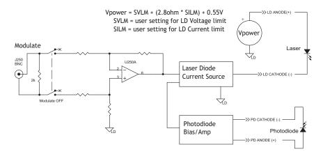
Figure 1.2: The laser diode drive circuitry (simplified).
