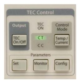
Figure 2.5: The TEC Control block.
