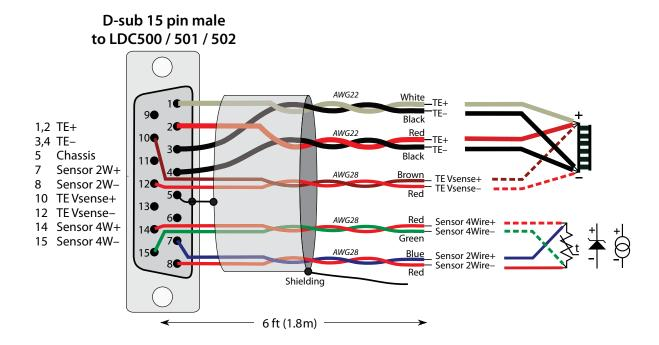
Figure 6.4: TEC cable with flying leads. SRS part number O500C2.
