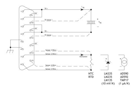
Figure 2.3: Wiring diagram for the TEC module. Pins 5 and 6 are internally connected to the chassis, and can be used for cable shielding. When the "dashed" connections are made from pins 10 and 12,  $V_{\rm TE}$  is a 4–wire measurement; otherwise, it is a 2–wire measurement. When the "dashed" connections are made from pins 14 and 15, the temperature sensor is read with a 4–wire measurement; otherwise a 2–wire measurement.
