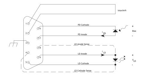
Figure 2.2: Wiring diagram for the Laser Diode. Pin 3 is internally connected to the chassis, and can be used for cable shielding. When the "dashed" connections are made,  $V_{\rm LD}$  is a 4–wire measurement; otherwise, it is a 2–wire measurement.
