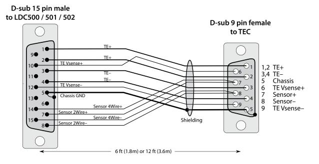
Figure 6.3: TEC cable with mating connector. SRS part number O500C4 (6 ft) or O500C6 (12 ft).
