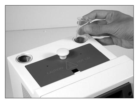
Figure 3. Mounting the glass Capillary Holders.
