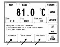
Figure 9. Use the Sample Buttons to flag important changes in the samples during the analysis.
