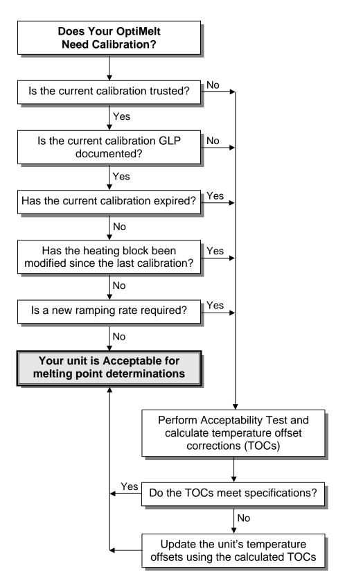
Figure 35. Temperature Offset Calibration Protocol.
