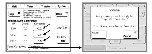
Figure 37. Enter and apply corrections.
