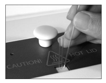
Figure 29. Loading capillaries into OptiMelt.
