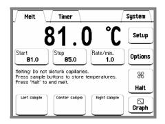
Figure 16. Sample buttons while ramping.
