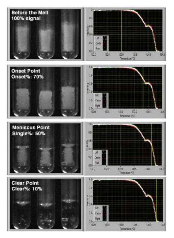
Figure 43. Melt Graphs provide a simplified representation of the melt process. Thresholds are assigned for the onset, meniscus and clear points, and are used by the digital image processor for automated determinations.
