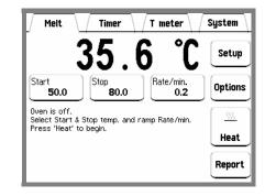
Figure 7. Melt Screen. Use the Start, Stop and Rate/min buttons to program the instrument. Follow the on-screen instructions to complete the analysis.
