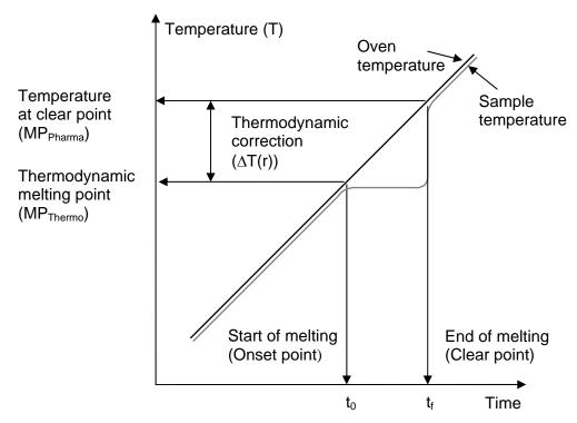
Figure 40. Graphical representation of the thermodynamic correction
