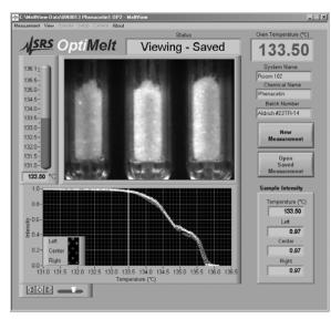
The sample images captured by the internal camera, and used by the Digital Image Processor, are also available for real-time transfer to a PC over the USB interface
