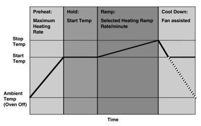
Figure 8. Analysis Heating Cycle.
