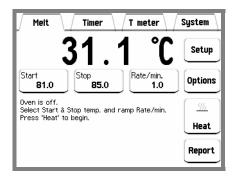
Figure 30. Melt Screen including Start temperature, Stop temperature and ramping Rate buttons required to program the OptiMelt.
