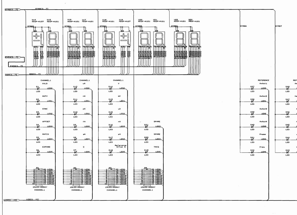
7 Segment LEDs, Display LEDs & Bar Graph Arrays
