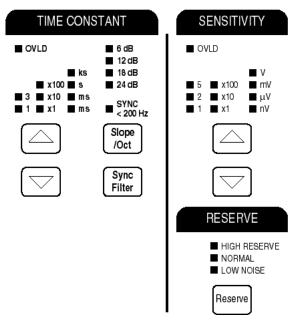
**[Sensitivity Up/Dn]** The [Sensitivity Up] and [Sensitivity Down] keys select the full scale sensitivity. The sensitivity is indicated by 1-2-5 times 1, 10 or 100 with the appropriate units.
