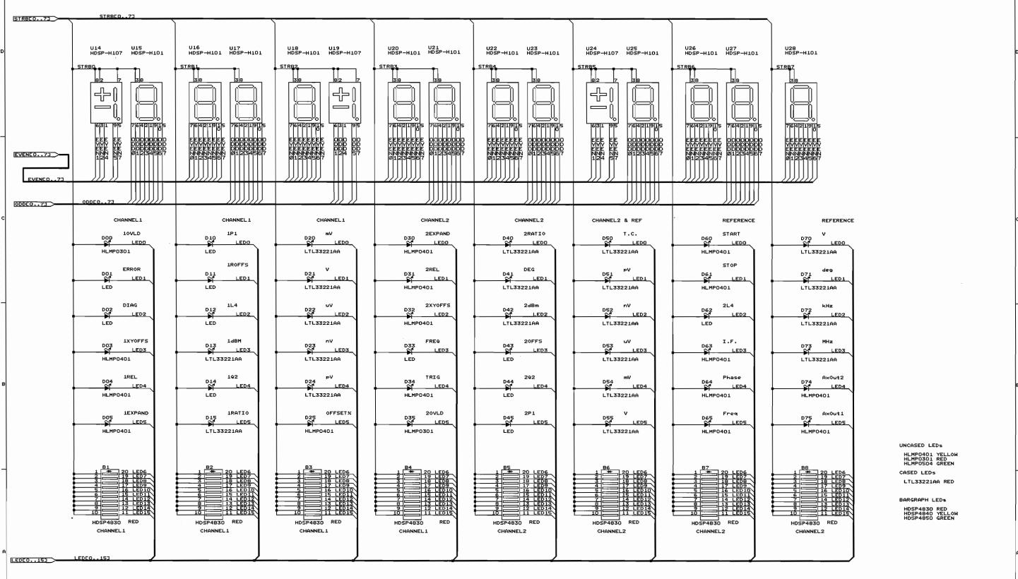
7 Segment LEDs, Display LEDs & Bar Graph Arrays
