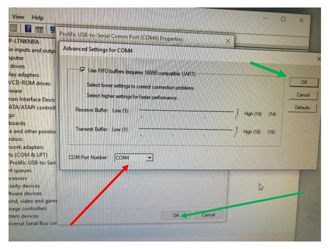
Check the Com Port Number (Red Arrow). If it's 9 or greater then change it to a port number (that you're not using) that is between 3 and 8. (1 & 2 are normally reserved for built in serial ports).
