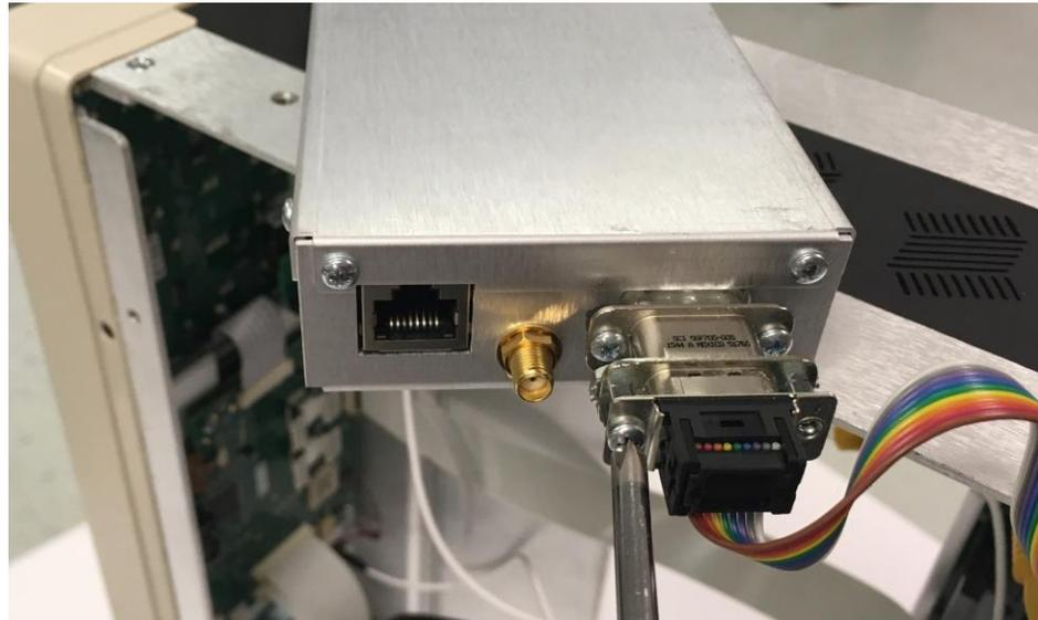
**13.** Slide the preamp enclosure back into the instrument chassis.
