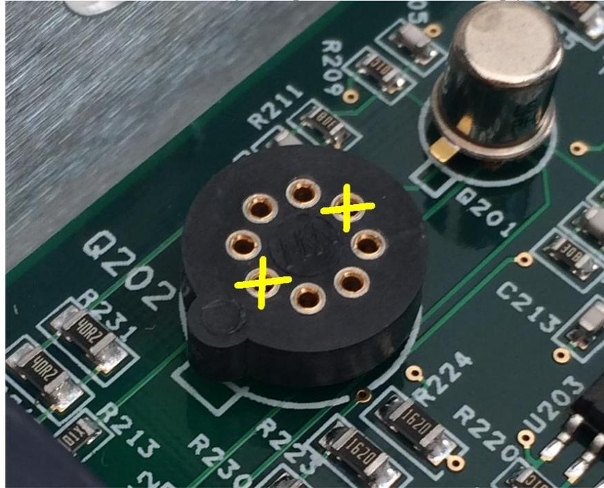
10. Install the replacement JFET, applying gentle pressure to fully seat all 6 leads into the socket receptacles. When fully seated, it should look like this:
