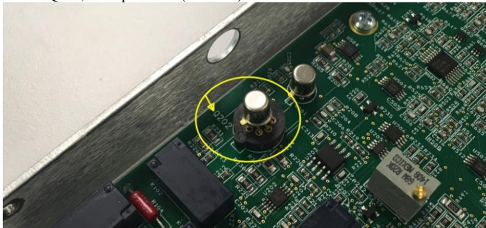
9. Carefully remove the old part from socket Q202 part (mark the old part first to avoid possible confusion). If necessary, trim and form the leads for the replacement JFET to match the removed part. Notice that two of the socket positions on Q202 are left empty—it is critical that the new part be installed with this same orientation, leaving the top and bottom contacts empty:
