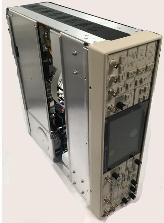
4. Disconnect the white coax cable, and the RJ-style modular cable, from the preamplifier enclosure. Do not attempt to disconnect the ribbon cable yet:
