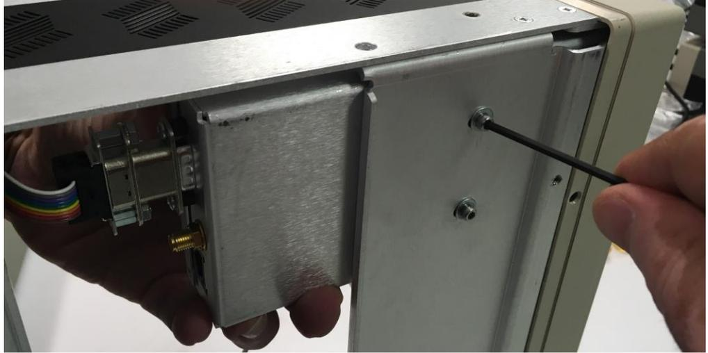
6. Carefully back the preamp enclosure out of the instrument chassis.
