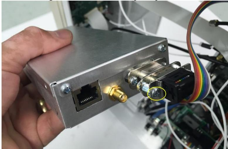
Once the screws are removed, disconnect the ribbon cable from the preamp.
