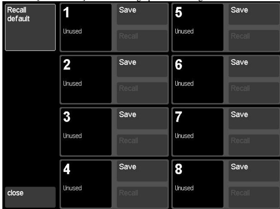
20. Touch the “Recall default” tile on the screen to restore default settings. Touch the “Confirm” tile on the screen that pops up to confirm restoring default settings.
