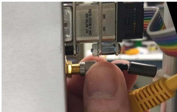
5. While supporting the metal preamplifier enclosure, remove the two #6 size hex screws securing the preamp to the chassis, using a 7/64 hex driver. Be careful to not lose the washers beneath each hex screw:
